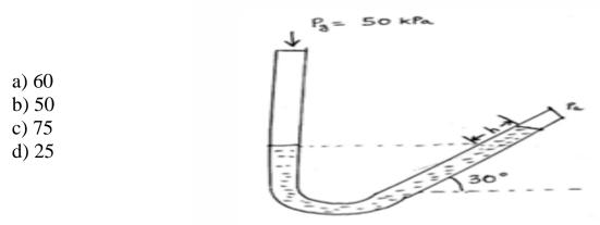
54- A single column manometer is connected to a pipe containing a liquid of specific gravity 0.75. Find the pressure in the pipe if the area of reservoir is 250 times the area of tube for the manometer reading. The difference in mercury level is 40 cm. On the left limb the fluid is upto the height of 20 cm.
